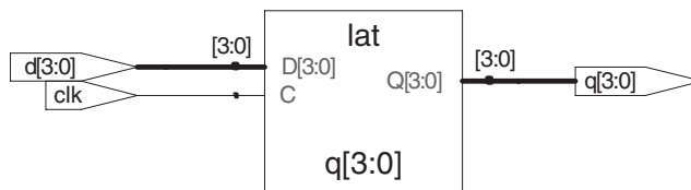
Figure 4.19 latch synthesized circuit
