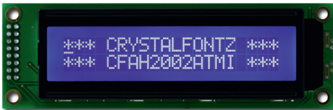
Figure e9.19 Crystalfontz CFAH2002A-TMI 20 \times 2 character LCD
